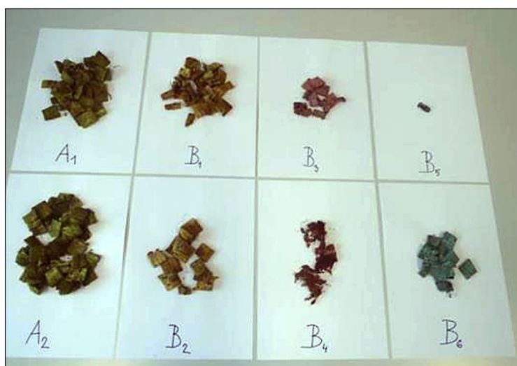
Figure 6. The sponge pieces after composting process
